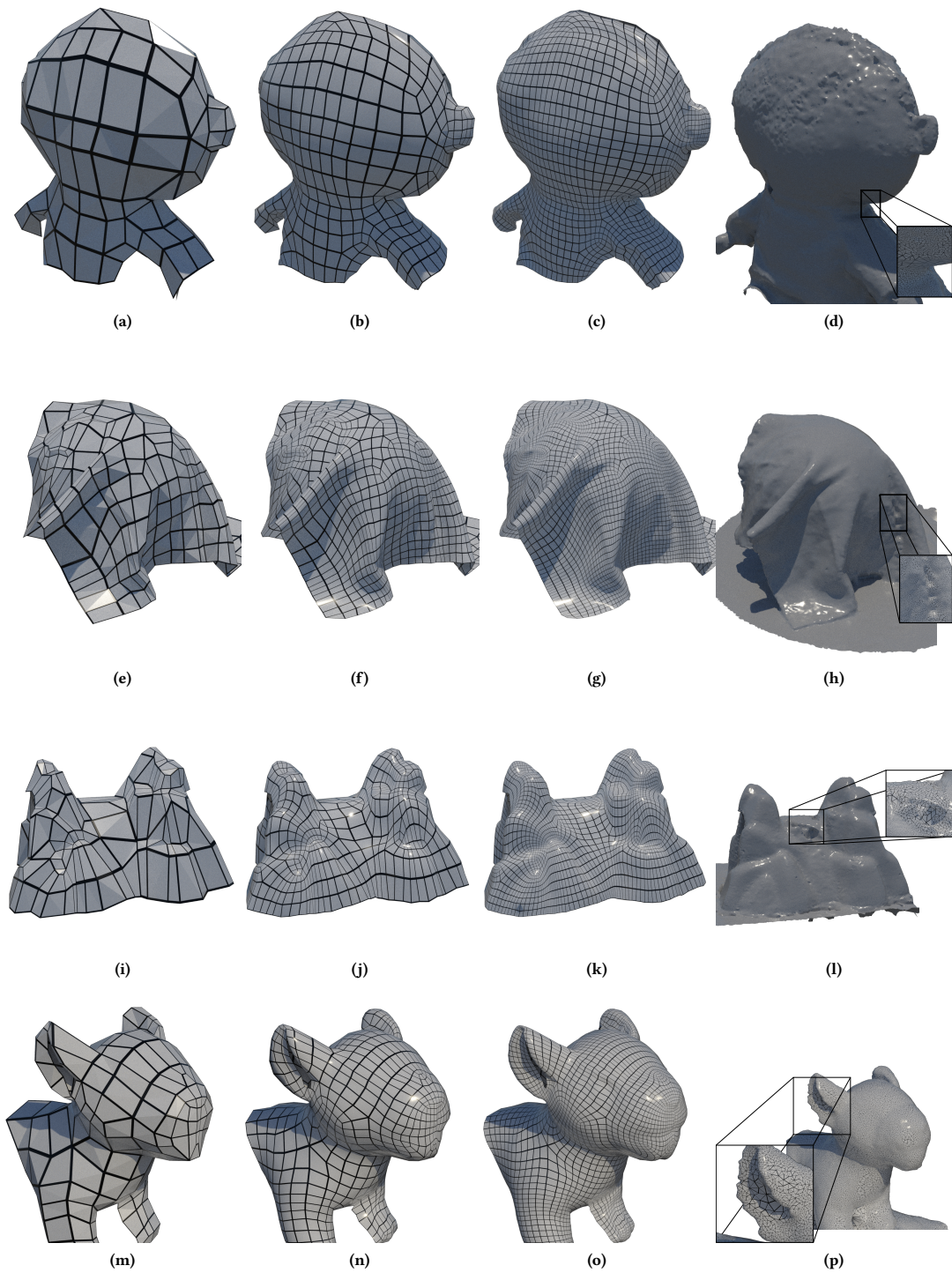
Figure 5: The difference in topology when using our tool (left three, from coarse to fine subdivision levels) and when using Meshroom (right-most images). Notice the high frequency, arbitrary topology shown in the insets of these images.
